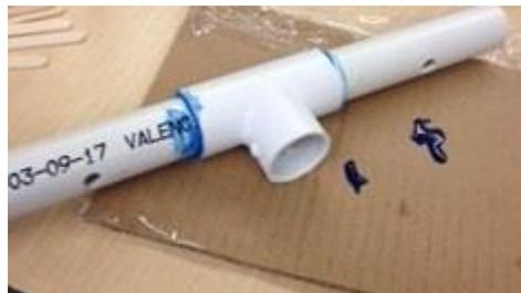
**Figure 9.** PVC adhesive on T-Shaped Section
