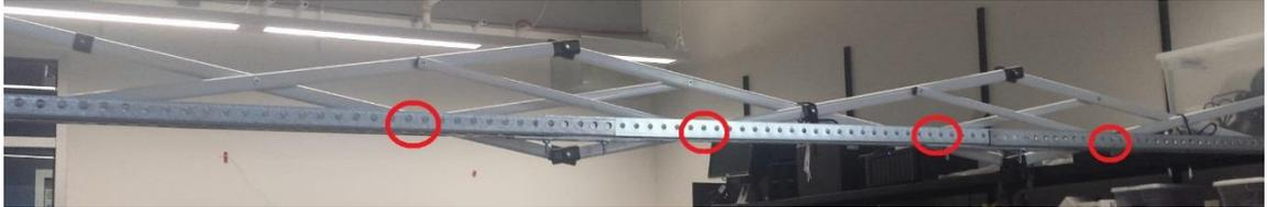
**Figure 7.** Zip Tie Locations to Secure Guide Rail
