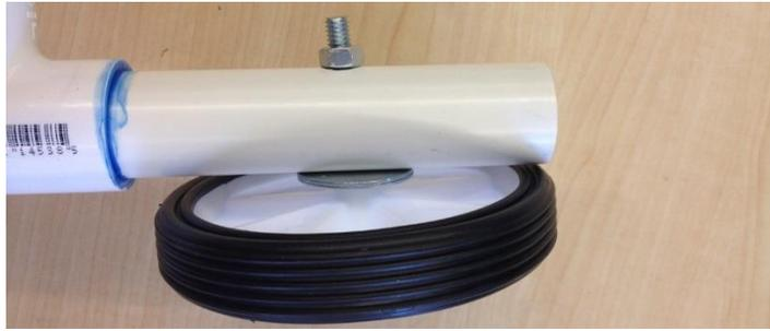
**Figure 10.** Wheel Washer Placement
