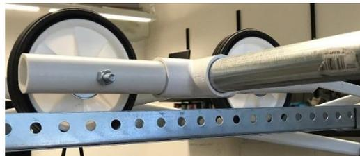
**Figure 12.** Wheels Inside Guide Rail
