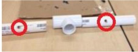
**Figure 8.** PVC Section (6") Drilling Locations
